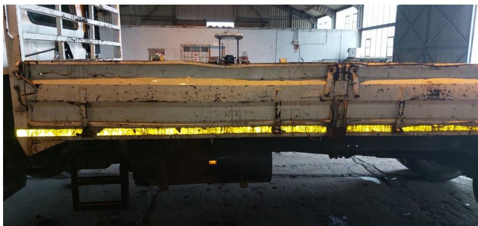
Image Above: Current condition of vehicle drop sides to be replaced.
